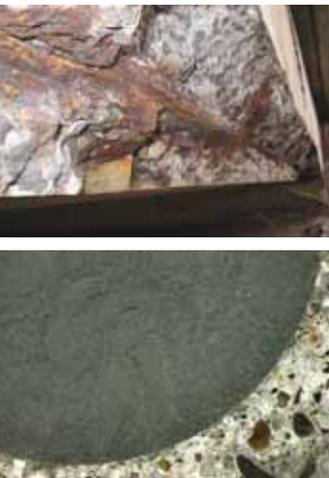
◀ After a comparable service life, the corrosion of the oxidized steel rebar has degraded the concrete around it, while the V•ROD rebar is intact and surrounded by healthy concrete.
